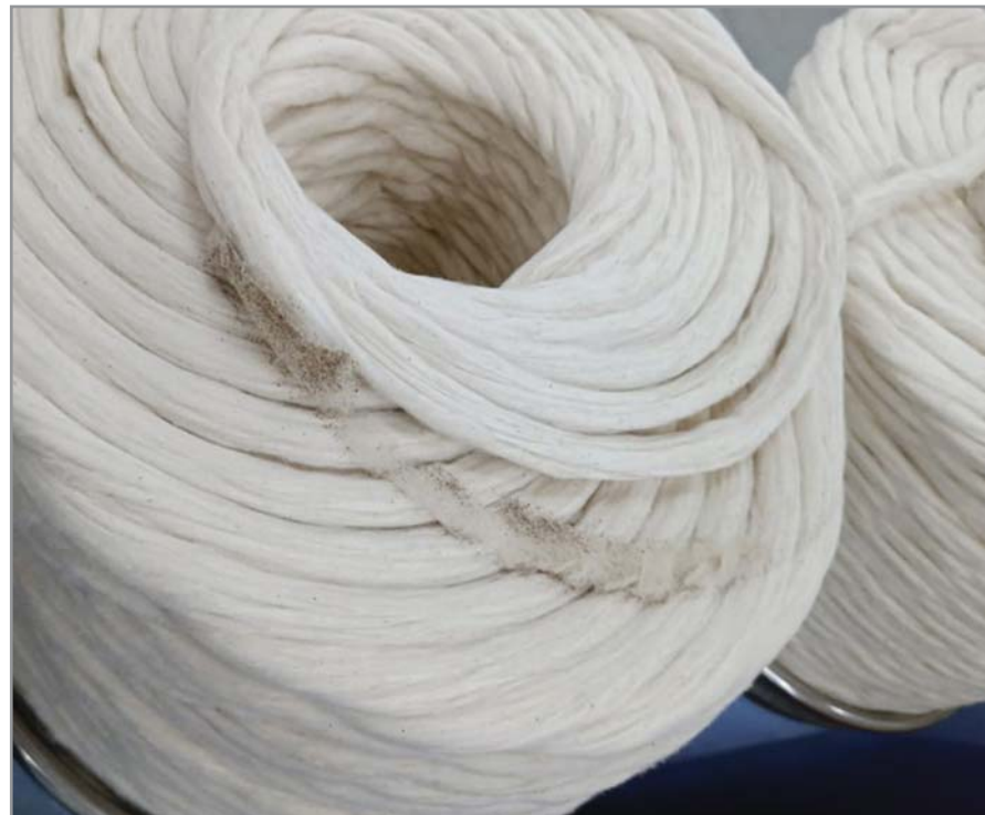
CLEANtube prevents trash particles and short fibres on the top sliver layer.
