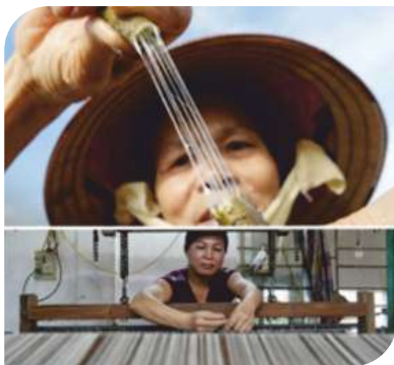
Fig 3b: Extraction of lotus stem fibre from the stems and formation of yarn.
